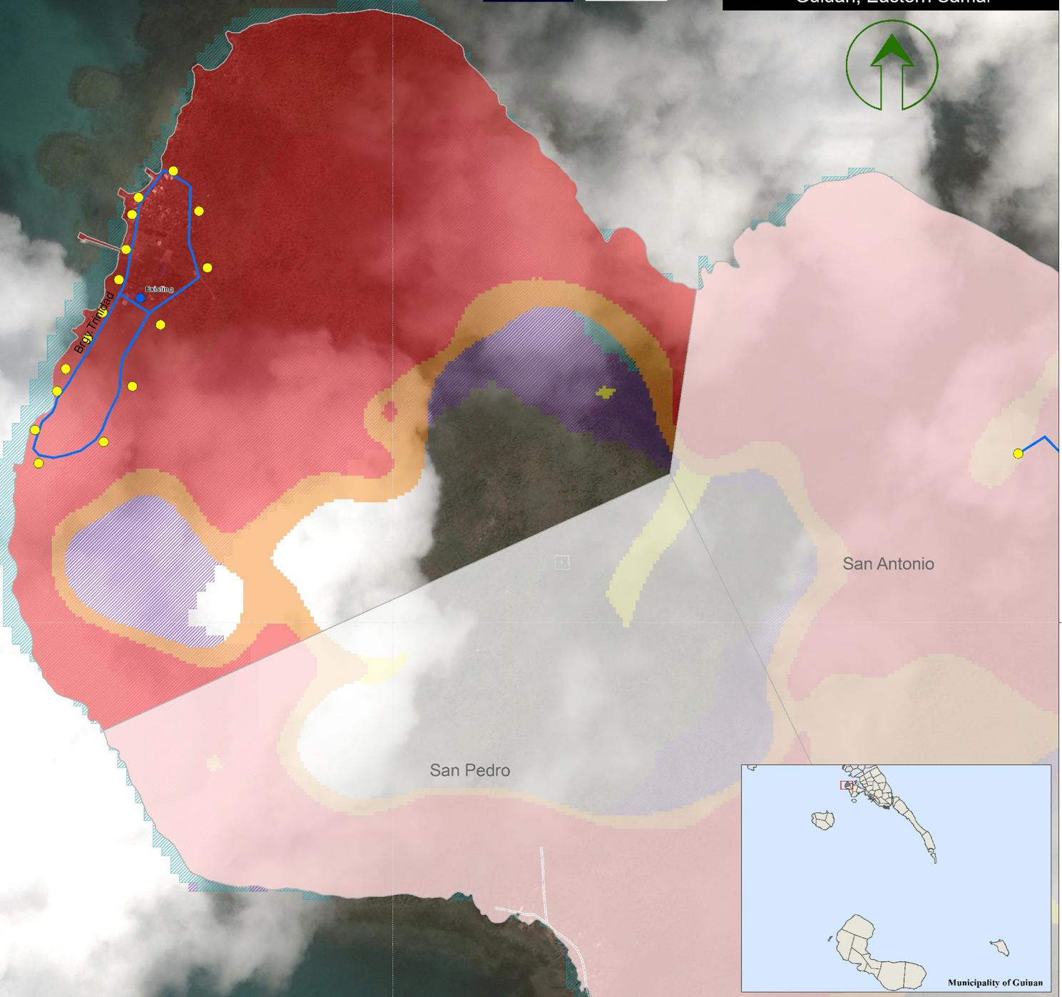
NOAH Multi-hazard Map is composed of a combination of landslide, flood, and storm surge hazards maps. Landslide hazard map identifies areas that may be affected by landslides; floods were simulated at a 100-year rain return scenario; and storm surge simulation was based on maximum storm tide heights of 5 meters.
