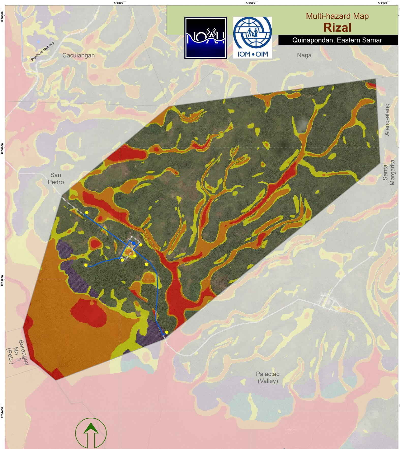
NOAH Multi-hazard Map is composed of a combination of landslide, flood, and storm surge hazards maps. Landslide hazard map identifies areas that may be affected by landslides; floods were simulated at a 100-year rain return scenario; and storm surge simulation was based on maximum storm tide heights of 5 meters.
