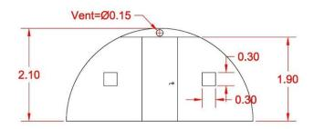
**Door Frame**: Galvanized Steel Pipe rec. Section 2cm x 4cm , Galvanized degree= 160-600 gm/m²
