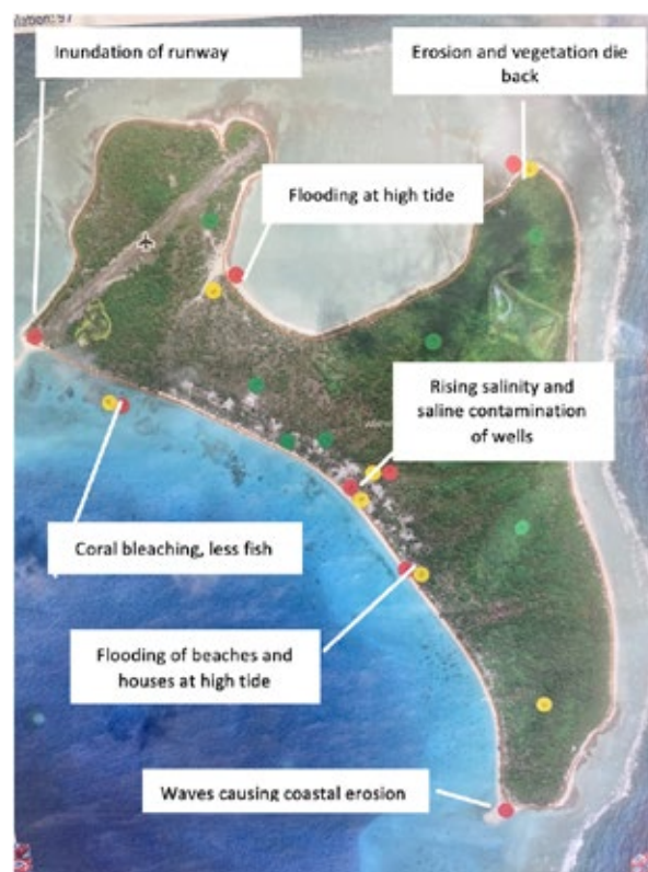
Figure 8: Impacts on infrastructure in Wotho
