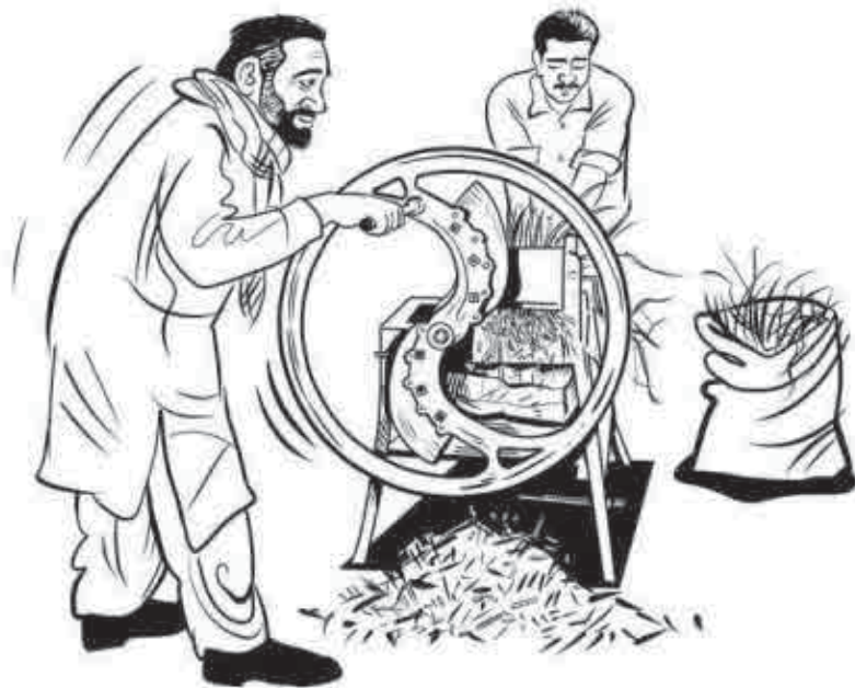
Fig 48: Producing short, chopped Fibres
