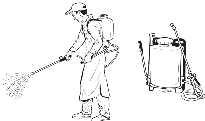
Fig 116: Agricultural back-pack sprayer: A very useful addition for misting (light spraying) of walls or blocks during the curing period. Application is easier than by hand, and gives a more uniform coverage.
