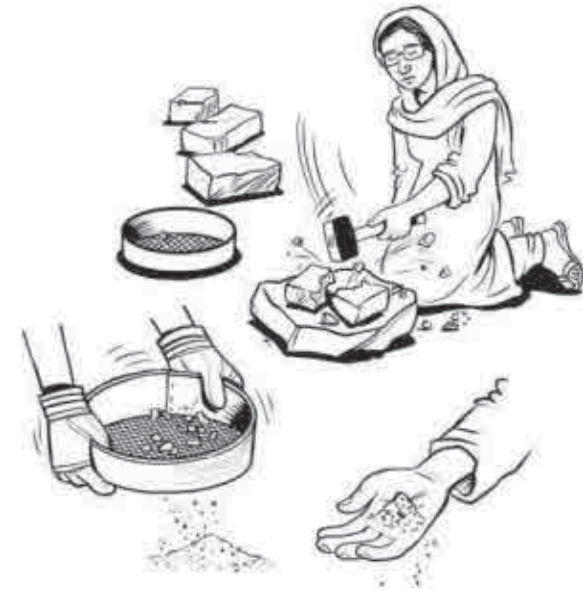
Fig 47b: The finer the pozzolan is ground, the more reactive it will be
