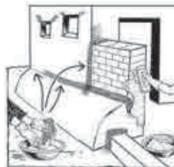
Fig 100: Reinforcing Joins to Reduce Risk of Cracking (Cracks in flood risk zones offer channels for water into the structure of the building and must be avoided).
