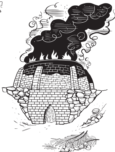
14a 2) Burning Limestone in a lime kiln
