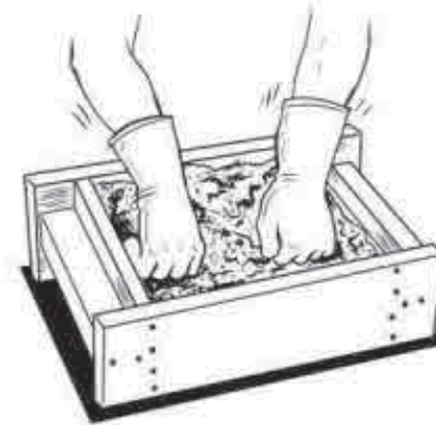
Fig 79 - Filling & compacting the block mould
