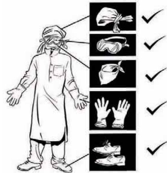
Fig 8: Wear Protective Clothing when working with Lime
