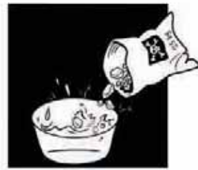
Fig 5: Always add Quicklime to Water, not water to Quicklime
