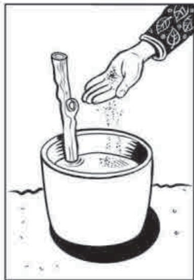
Fig 111: Add small amounts of earth pigments for colouring limewash. Mix well. (Mix enough quantity to cover an entire wall for colour match)
