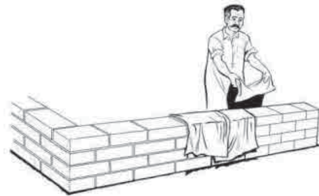
Fig 86: Keep newly laid block walling dampened and shaded throughout the work, to stop the mortar drying out too quickly
