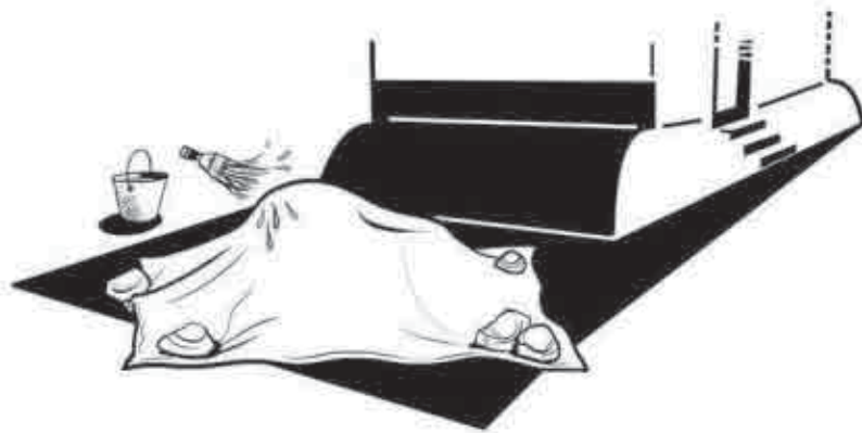
Fig 75: Cover any lime putty based mixtures from drying sun or rain, if they are not being used immediately
