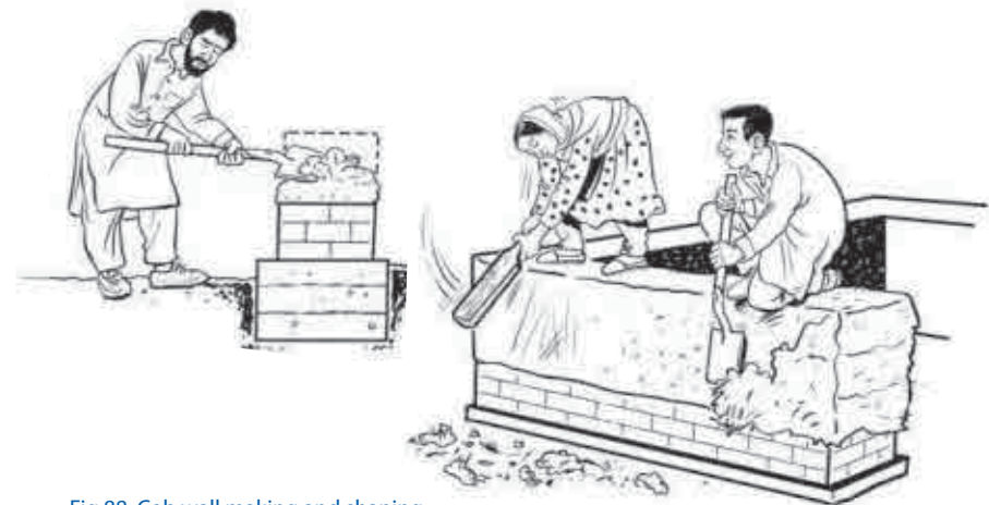
Fig 88: Cob wall making and shaping
