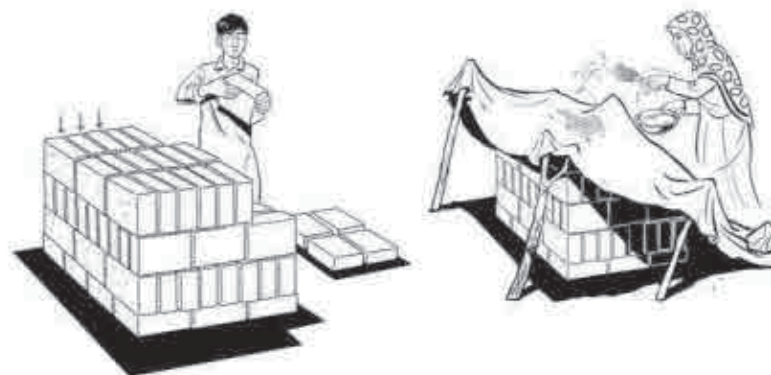
Fig 84: Stacking, curing and storage of blocks
