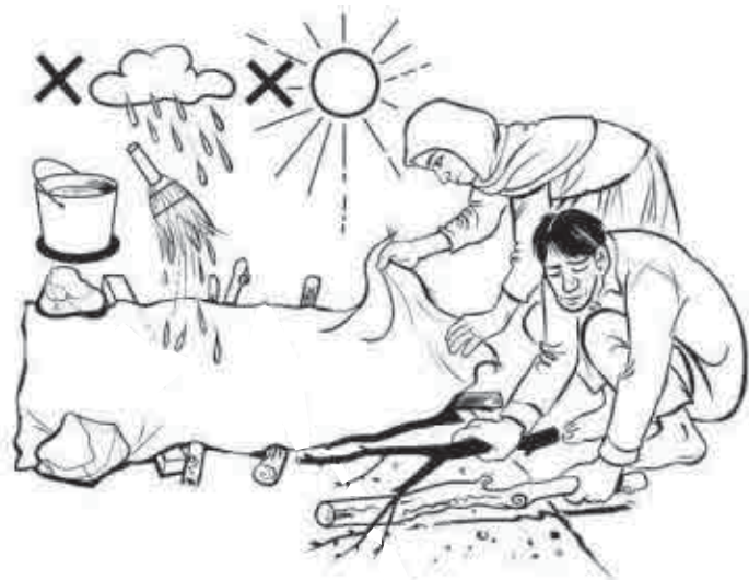
Fig 104: Curing of Floor Screeds: Keep shaded and lightly dampened for a minimum of 1 week, preferably 4 weeks
