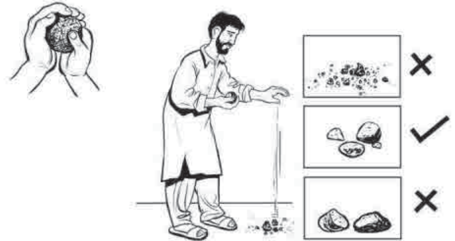
Fig 76: Ball Drop Test for Optimum Moisture Content
