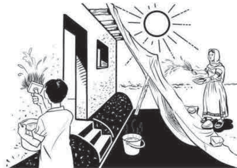
Fig 99: Cure for 28 days - keep shaded and dampened
