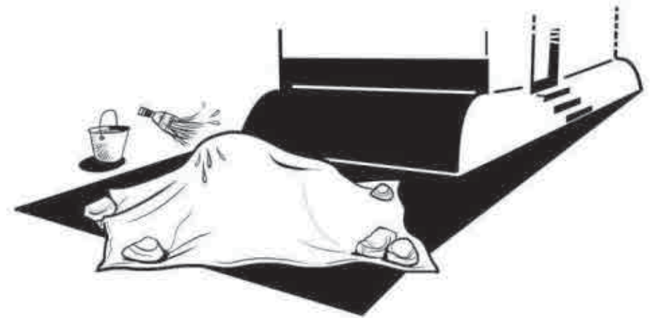
Fig 96: Storage and protection of mixes
