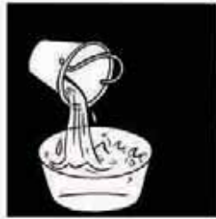
Fig 5: Always add Quicklime to Water, not water to Quicklime
