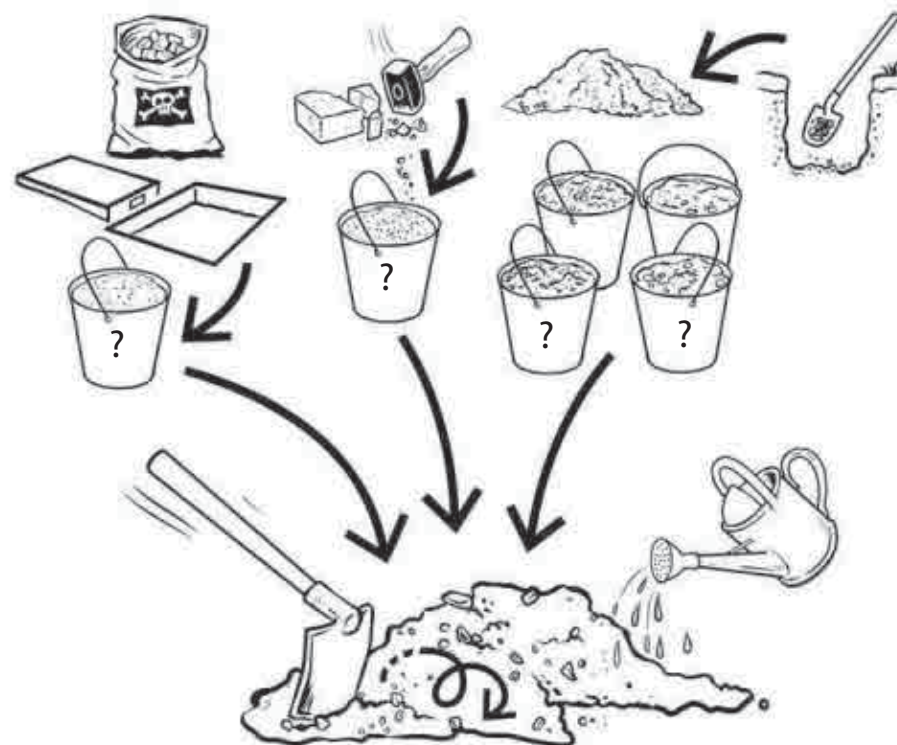
Fig 91: Subject to testing, a trial mix for low clay soils could be : 1QL (or 2LP) : 3 finely sieved pozzolan : 4 or more parts of sandy soil, plus fibres and just enough water to make the mix sticky and workable
