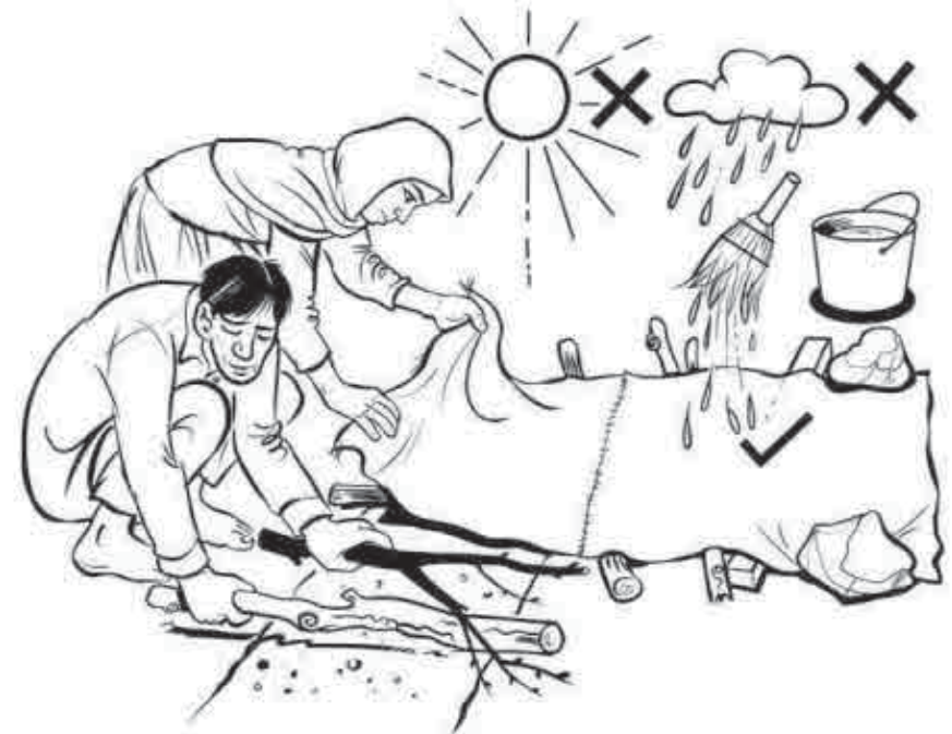
Fig 74: Keep all foundation work very well cured for maximum strength and hydraulic set
