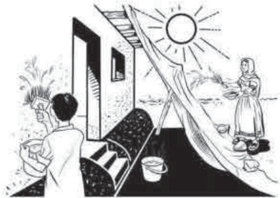
Fig 87: Protect new walls and mortar from drying out too quickly. Keep shaded and regularly dampened
