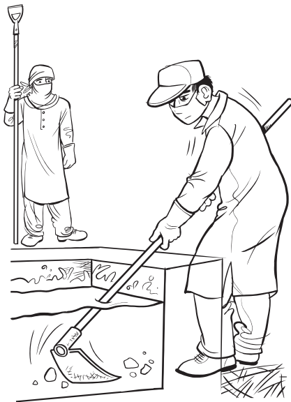
Fig 32: Use long handled Hoes to keep the quicklime lumps moving and to ensure all quicklime is fully submerged under water at all times
