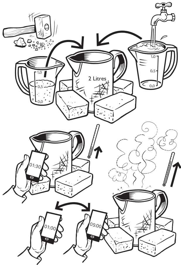
Fig 21: Lime Reactivity Test
