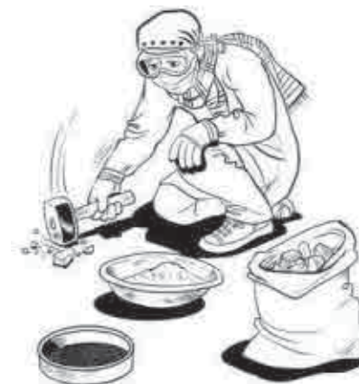
Fig 15: Crushing Quicklime to Powder
