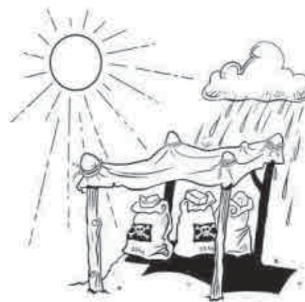
Fig 14b: Protection of Quicklime : Protect the Quicklime from Moisture
