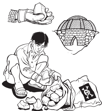
14a 3) Bagging quicklime with gloved hands into watertight and airtight bags
