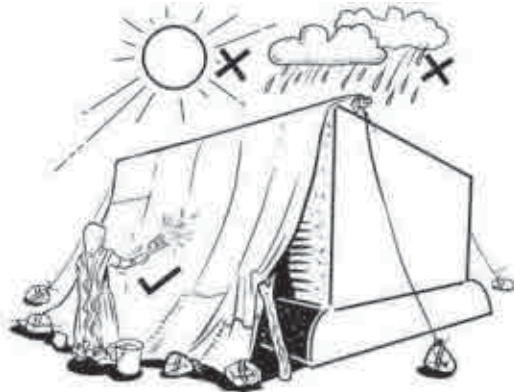
Fig 94b: Providing shade for all lime stabilized work
